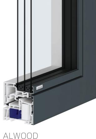
Timber/aluminium window with best values due to massive thickness of 101 mm. HYBRID frame with HYBRID thermal insulation and serial triple glazing with Ug 0.5 W/m2K.
